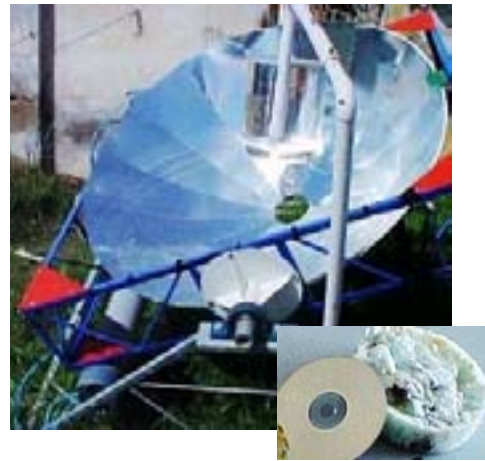
Solar melters can compress a full safety box—including syringes and needles—into a cake the size of a compact disc.
